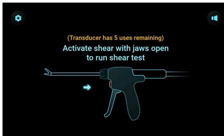
Note: if the remaining use of the Transducer is less than 10, the following image will be displayed. Please pay attention to the number as the Transducer needs to be replaced when the number is zero:
