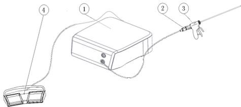
Figure 1 Composition Drawing of the Ultrasound Surgical Equipment
